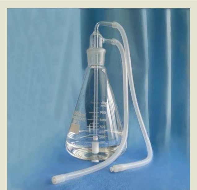
A container of water that is connected to an ozone generator through tubing creates Ozonated water
